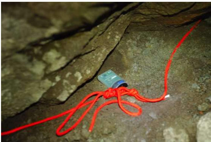
Figure 1. Sample MSH01, showing temperature/light data logger at fumarole entrance.
