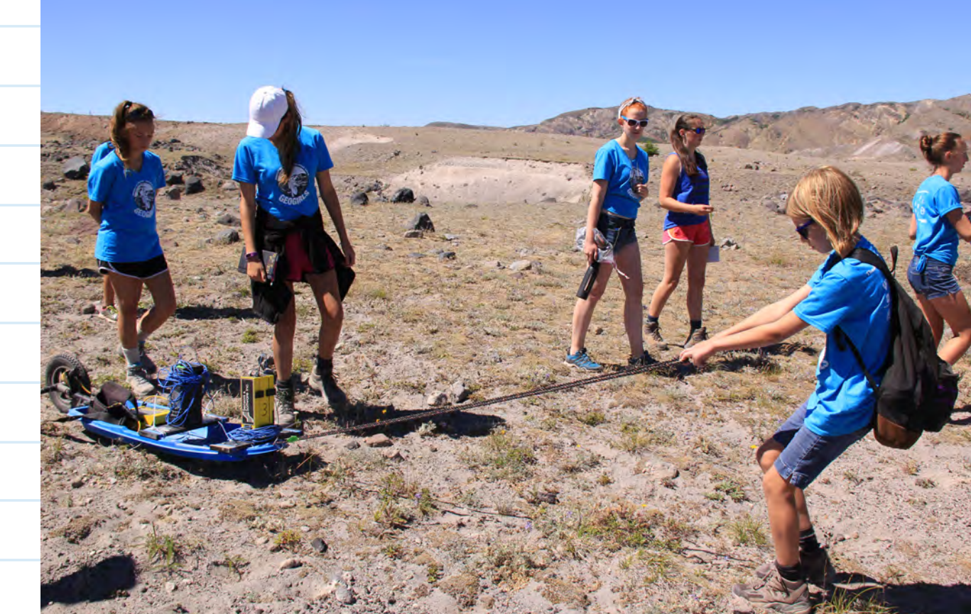
Figure 7 (left): On the Pumice Plain, GeoGirls take turns collecting data using a GPR device assembled by field researchers from Boise State University.
